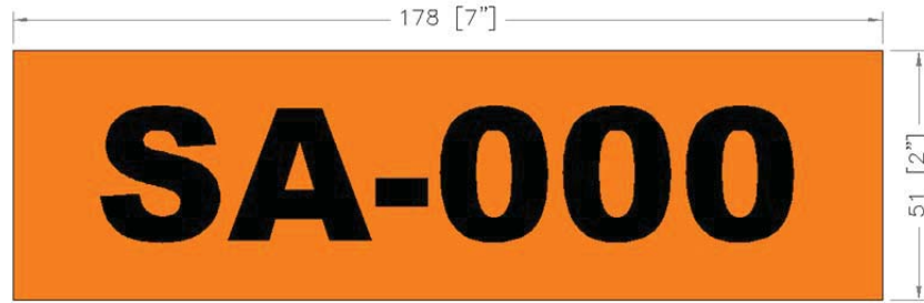
Figure-2 Equipment Label (Example)
