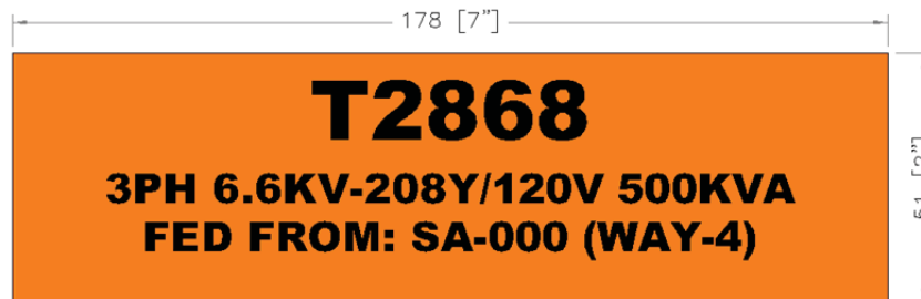
Figure-9 Transformer Information Label (Example)
