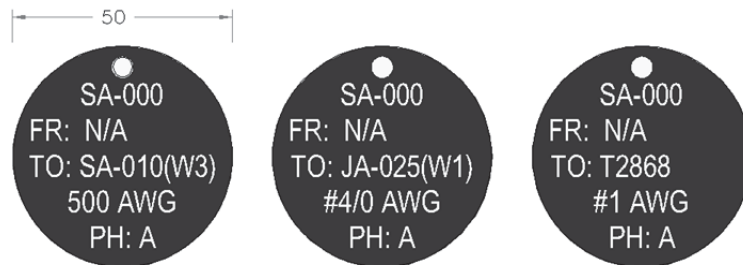
Figure-5 Primary Cable Identification Tags (Example)
