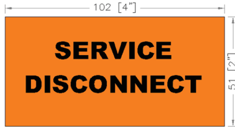
Figure-15 Service Disconnect Label
